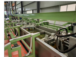
Air Underwater Test
