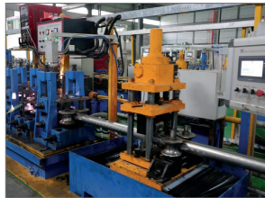
Welded Bead Removing
