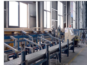
Offline Eddy Current Test
